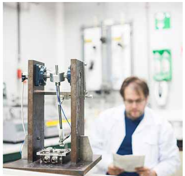
Schematic drawing and picture of the new test setup which allows to test samples under both shear and axial (pull) shock mode.
