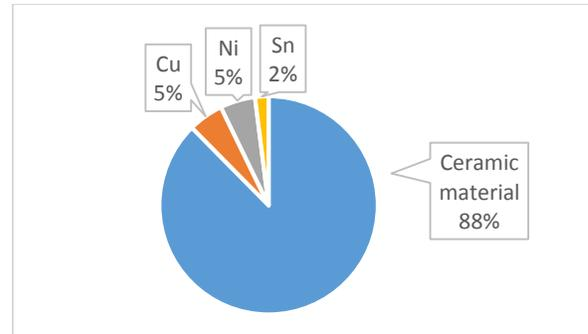
Figure 6: Weight percentages for the main materials in a 0603 ceramic capacitor
