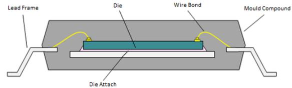
Figure 3: Example of a gull-wing leaded active component
