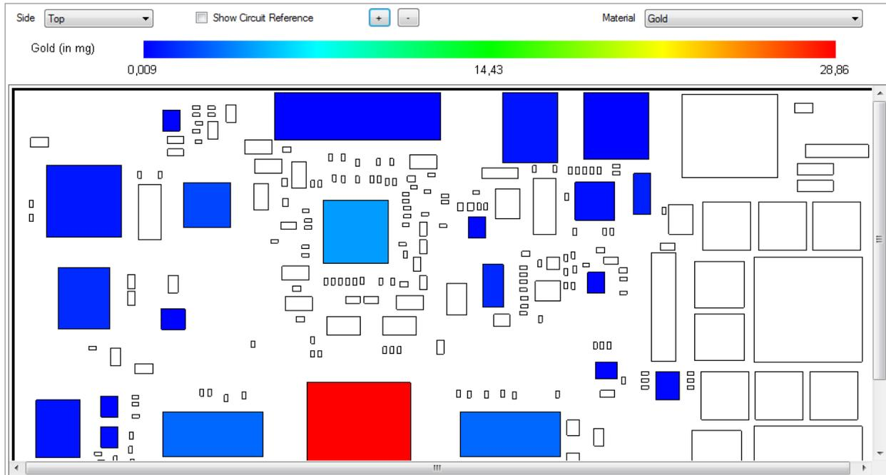
Figure 7: Gold distribution on a printed board assembly
