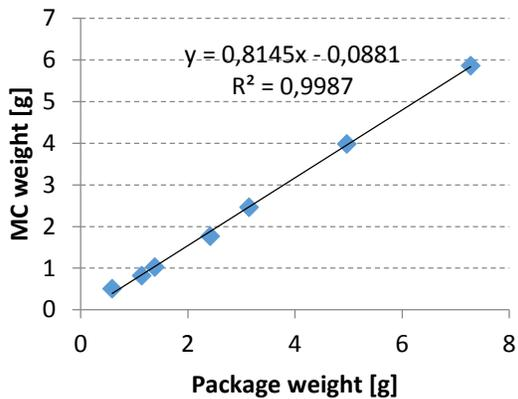
Figure 4: Mould compound weight vs total package weight for PLCC packages
