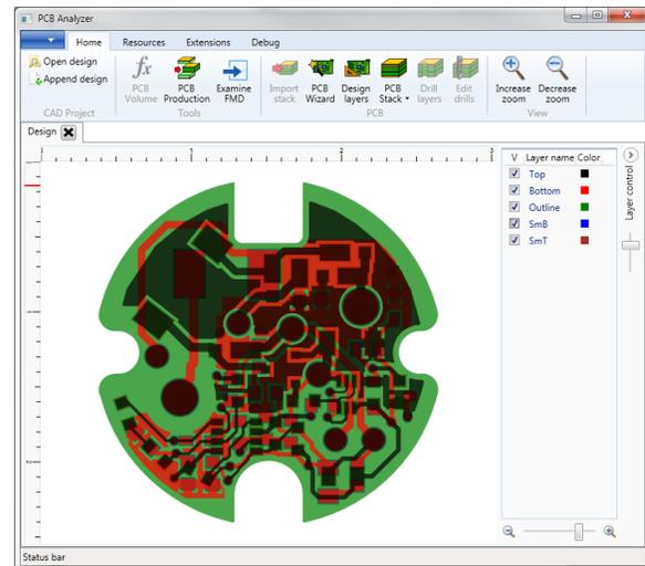
Figure 2: Philips LED lamp driver PCB design loaded in the prototype application
