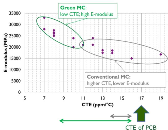
Fig. 1. Correlation between the mold CTE and mold stiffness for a wide range of commercially available mold compounds. The graph also indicates the larger gap between the CTE's of the PCB and the green mold compounds
