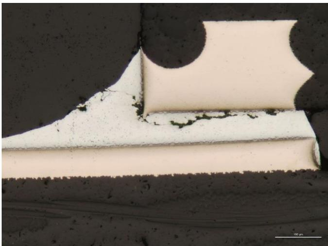
Fig. 9. Cross-section of SAC305 soldered QFN component with 7 ppm/°C mold compound and wettable flanks
