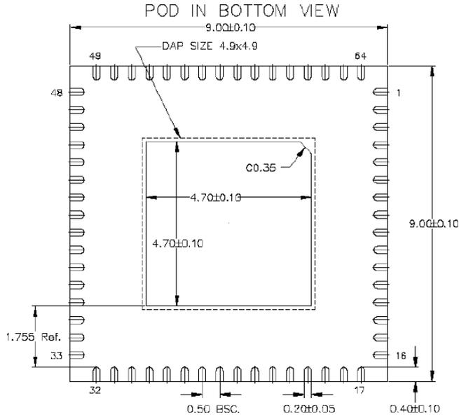
Fig. 2. Package outline drawing for the QFN package used in this BLR analysis
