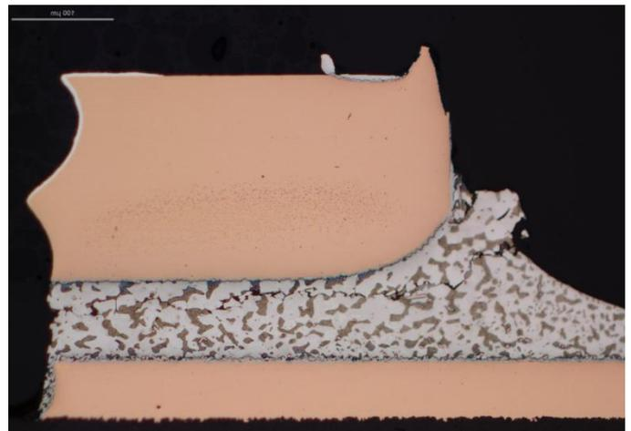
Fig. 7. Cross-section of SnPb soldered QFN component with 12 ppm/°C mold compound and non-wettable flanks
