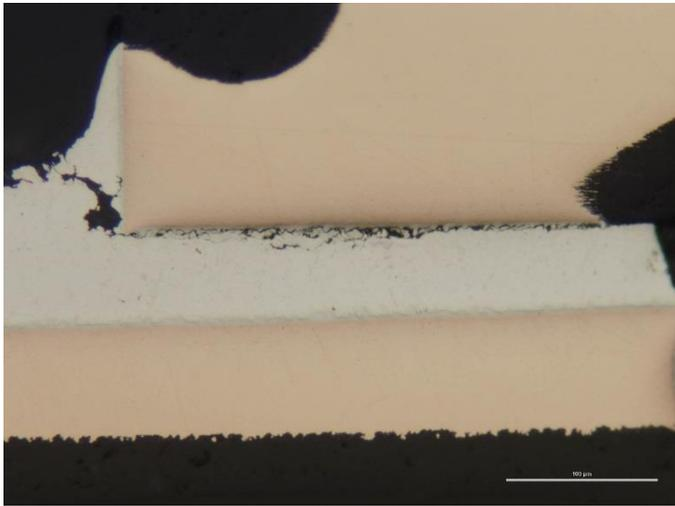
Fig. 8. Cross-section of SAC305 soldered QFN component with 7 ppm/°C mold compound and non-wettable flanks
