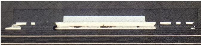
Fig. 3. Cross-section of QFN component soldered to a 2.4 mm thick PCB
