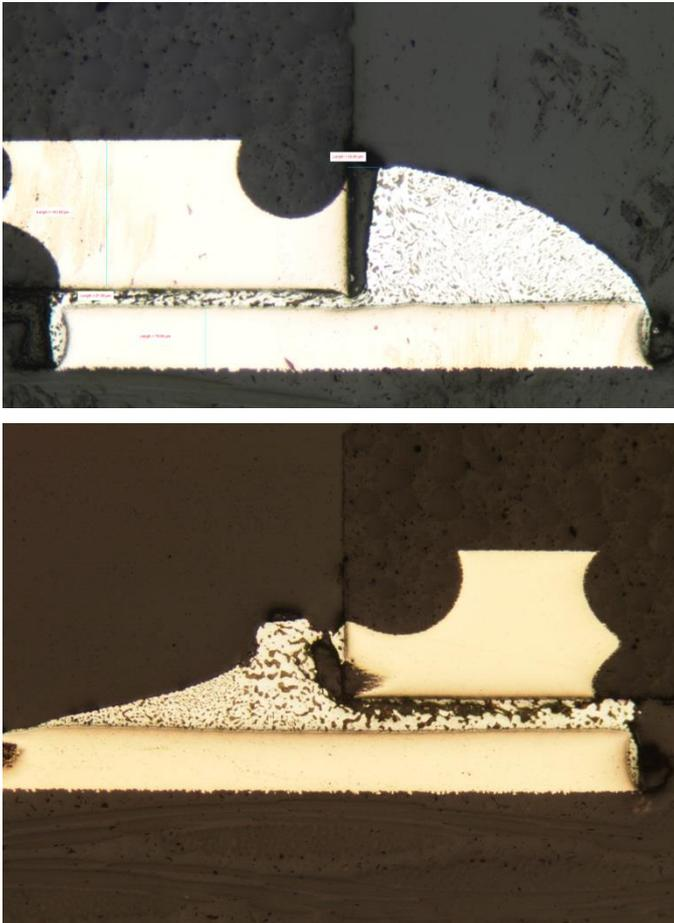
Fig. 5. Cross-section of SnPb soldered QFN component with 7 ppm/°C mold compound and non-wettable flanks
