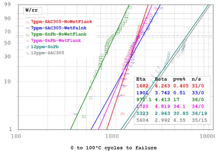
Fig. 4. Weibull distribution of 6 tested QFN64 solder assemblies.
