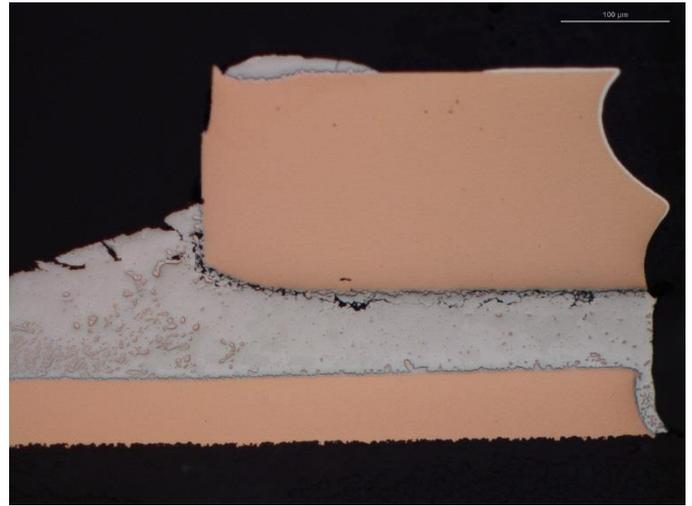
Fig. 10. Cross-section of SAC305 soldered QFN component with 12 ppm/°C mold compound and non-wettable flanks
