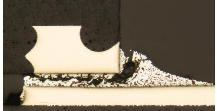
Fig. 6. Cross-section of SnPb soldered QFN component with 7 ppm/°C mold compound and wettable flanks
